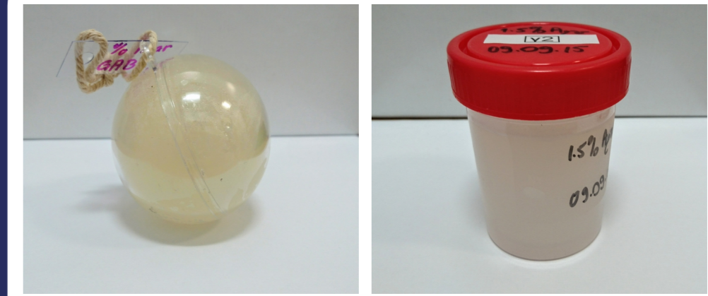
Fig6 - Spherical spectroscopy phantom (left) and plain agar phantom for calibration (right)
