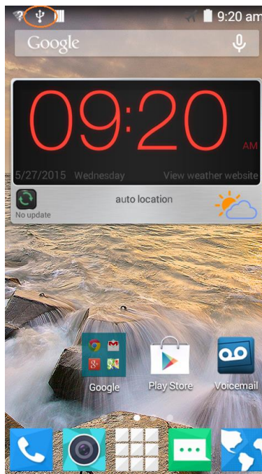
Figure 79 - When connected to PC, a USB icon should be visible near top of screen (in orange circle).
